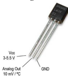
Gambar 3. Sensor LM35
